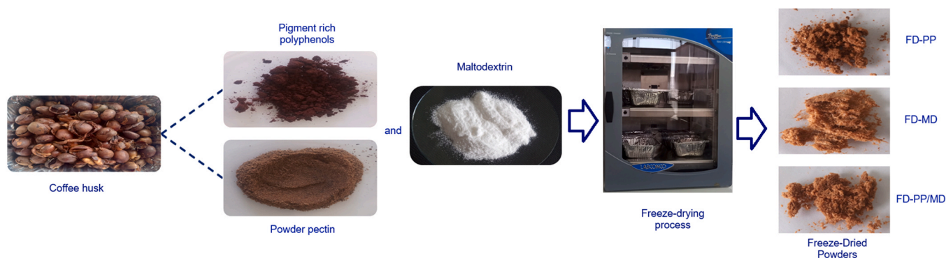
Fig. 1. Schematic representation of the microencapsulation process of pigment rich polyphenols using powder pectin (PP), maltodextrin (MD), and a powder pectin–maltodextrin (PP/MD) mixture as wall materials.
